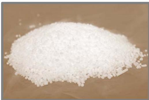
Solid carbon dioxide pellets remove not only the surface contaminant but also substrate material, adding a profile. Baking soda, by contrast, does not profile or remove substrate material. The only thing baking soda removes is the surface contaminant or coating that needs to be removed.
