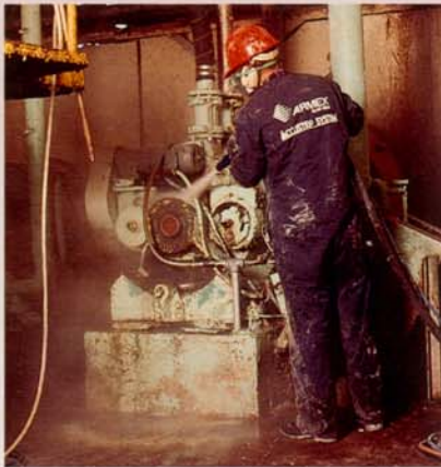
▲ Grease and paint removed from wet end refiner while operating
