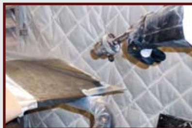
ing larger panels such as hoods, trunk lids and roofs, a lower pressure range of 40-50 psi is recommended. Increasing the stand-off distance will also lower the pressure impact on the surface. If panel flexing is observed, adjust the psi and stand-off distance as required.
